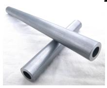
Made by rifling standard DOM tubing, our Rifled Tubing has any number of uses, ranging from exotic fluid-flow applications to inexpensive muzzle-loader barrels. With an outer diameter of <sup>7</sup>/<sub>8</sub> inch and a wall thickness of <sup>3</sup>/<sub>16</sub> inch, the bore is about .50-caliber. Available in lengths from 6 inches to 46 inches.
