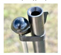
Barrels are button-rifled with a 1:24 inch twist rate, and feature a generous 60-degree muzzle crown that acts as an integral loading funnel.
